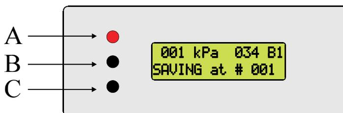
The display will show: "SAVING AT # XXX", where 001 is the memory position where the value is stored (between 1 and 100). If the value is not to be stored just push A. The registered maximum value is then erased from the display.
