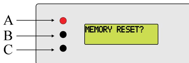
The text "MEMORY RESET?" is shown on the upper line. To erase, push **C** twice.
