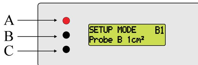
The display will show the text "SETUP MODE" on the upper line, and on the lower line "PROBE B 1cm<sup>2</sup>". With **C** button the size can be chosen between 0.5 cm<sup>2</sup> and 2 cm<sup>2</sup>.
