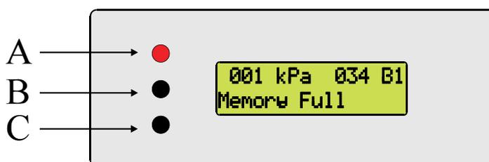
e/ When overloading the Algometer (more than 2000 kPa with probe 1 cm<sup>2</sup>) a buzzer will sound and the text "WARNING OVERLOAD" will be shown on the display. The warning text is erased by pushing **A**.
