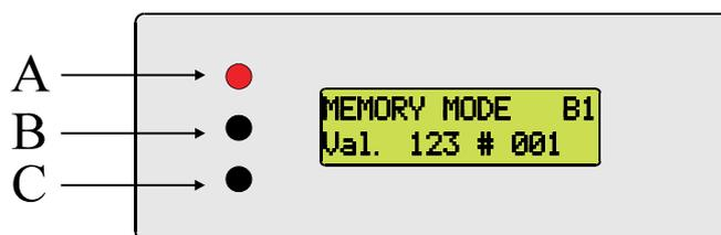
The text "MEMORY MODE" is shown on the upper line. At the same time the text "VAL. XXX #001" will be shown on the lower line, which means VALUE XXX in memory position 001. By pushing **C** the memory positions will be stepped forward to the last stored position. By pushing **B** the memory positions will be stepped backwards. If it is impossible to step forward from position no. 1 there is nothing stored in the memory.
