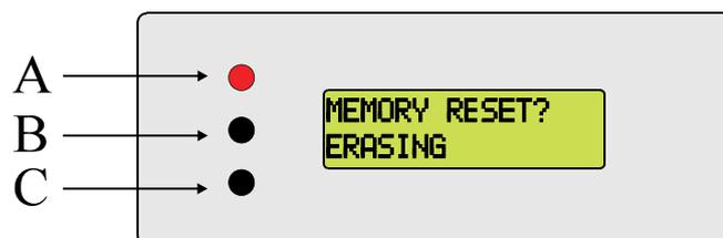
The text "ERASING" is shown on the lower line. If no erasing is desired just simply push **A**.
