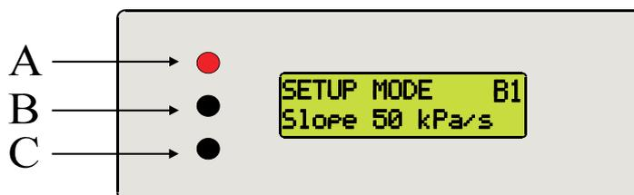
On the lower line the text "SLOPE 10 kPa/s" will be shown. Using **C** the desired slope between 10 kPa/s and 50 kPa/s can be chosen in 5 intervals. When the desired value is achieved press **A**. The adjusted value is indicated on the upper line to the right according to the following:
